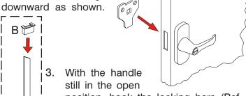
still in the open position, hook the locking bars (Ref. No. 10) to the locking cam (see "A" at left). Then, hold the lock bars in position while sliding the nylon lock bar guide inserts (Ref. No. 13) over
