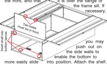
more easily slide into position. Attach the she securely by bolting the bottom to the frame sill with two bolts and nuts.
