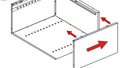
6. Attach the sill (Ref. No. 5) to the sides. Place nut loosely on each of the studs and slide the ends of the sill into the slots on both sides of the unit.
