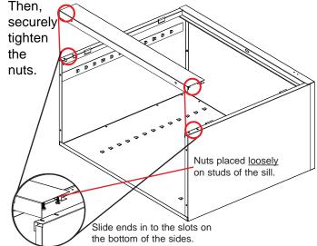
7. Place rear flange of the bottom (Ref. No. 6) into the bottom lances of the back. The flange with two holes should face
