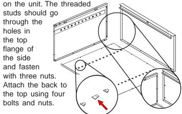
5. Attach the right side (Ref. No. 3) to the back in the same manner as you did in step 3, again making sure that the flange is around the back and that the lances on the shelf adjustment strips are pointed in the same direction as those on the back and left side. Push the side panel up so the studs in the top go through the holes in the top flange of side and fasten with three nuts.
