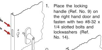
2. Turn the handle to the open position, and place the locking cam (Ref. No. 10) over the square shank of the door handle. The latch must be facing downward as shown. Then place the locking cotter pin (Ref. No. 12) through the hole of the square shank as shown at right.
