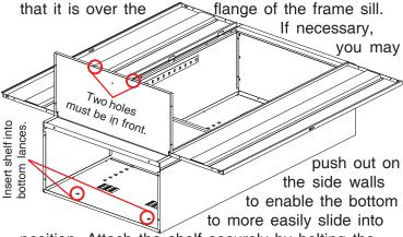
position. Attach the shelf securely by bolting the bottom to the frame sill with two bolts and nuts.
