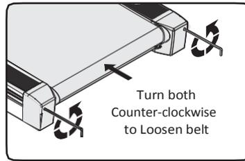
**CAUTION: DO NOT** tighten more than 2 full turns on each side. Over tensioning the belt can cause unnecessary friction and wear and tear on the belt, motor and electronics.
