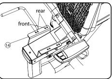
C. Install four *M8x15L Bolts (17)* through the *Seat Mount (14)* into the *Seat Bottom (9)*. Be sure to install all four bolts before tightening.
