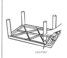
Lay top shelf (with handle) ribbed side up on a smooth surface. Push all 4 short Legs (6.5") onto leg posts
