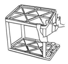
Position center shelf (with 8 leg posts) ribbed side up, over the 4 legs and insert leg posts into legs. Using a rubber Mallet, firmly hammer center shelf into legs until all 4 legs are seated (flush) against the surfaces of both shelves.
