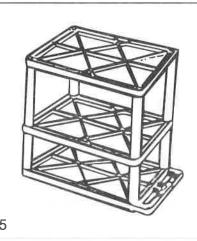
Position bottom shelf, ribbed side up. over the 4 legs and insert leg posts into legs. Using a rubber mallet, firmly hammer bottom shelf into legs until all 4 legs are seated (flush) against the surfaces of both shelves.
