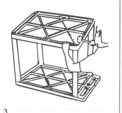
Position bottom shelf with 4 leg posts, ribbed side up, over the 4 legs and insert leg posts into legs. Using a rubber Mallet, firmly hammer bottom shelf into legs until all 4 legs are seated (flush) against the surfaces of both shelves
