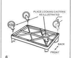
Push the four casters firmly into the holes in each corner of the bottom shelf. Important: Casters must be fully seated. Tap firmly with rubber mailet to properly seat casters. Turn your A/V CART right side up. It is now ready for use.
