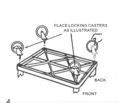
Push the four casters firmly into the holes in each corner of the bottom shelf. Important: Casters must be fully seated. Tap firmly with rubber mallet to properly seat casters. Turn your A/V CART right side up. It is now ready for use.
