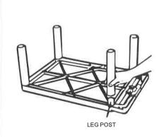
Lay top shelf (with handle) ribbed sideup on a smooth surface. Push all 4 Long Legs (17.5") onto leg posts
