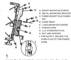
Insert the 3 receptacle power tap into the cavity
