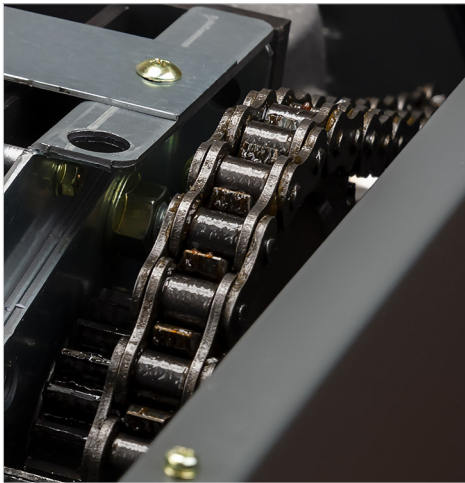
Powerful chain-driven motor provides slip-free performance.
