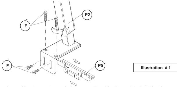
3.) Loosen the two Allen Recess Screws in the rear section of the Support Post's (P2) table clamp. Next, loosen the two Allen Recess Screws in the top section. Slide the Support Post (P2) onto the back of the table you will be using. Tighten the two top Screws (E) using Allen Wrench (C) untill the Support Post is firmly in place. Tighten the two Screws (F) in the rear of the clamp to lock the unit in place. See illustration #2.
