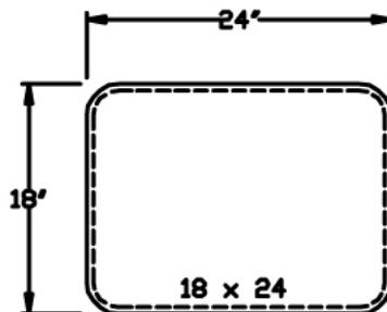
**Millennium™ Shell:** One-piece shell is injection molded from special high impact, blush resistant polypropylene plastic with and antistatic additive. Textured surface is etched to provide a non-slip surface while assisting in maintaining like-new appearance. Flanged opening in the back adds strength and ventilation. The underside of the shell is molded with an advanced rib pattern transferring weight directly to the frame. The shell is attached to frame with
